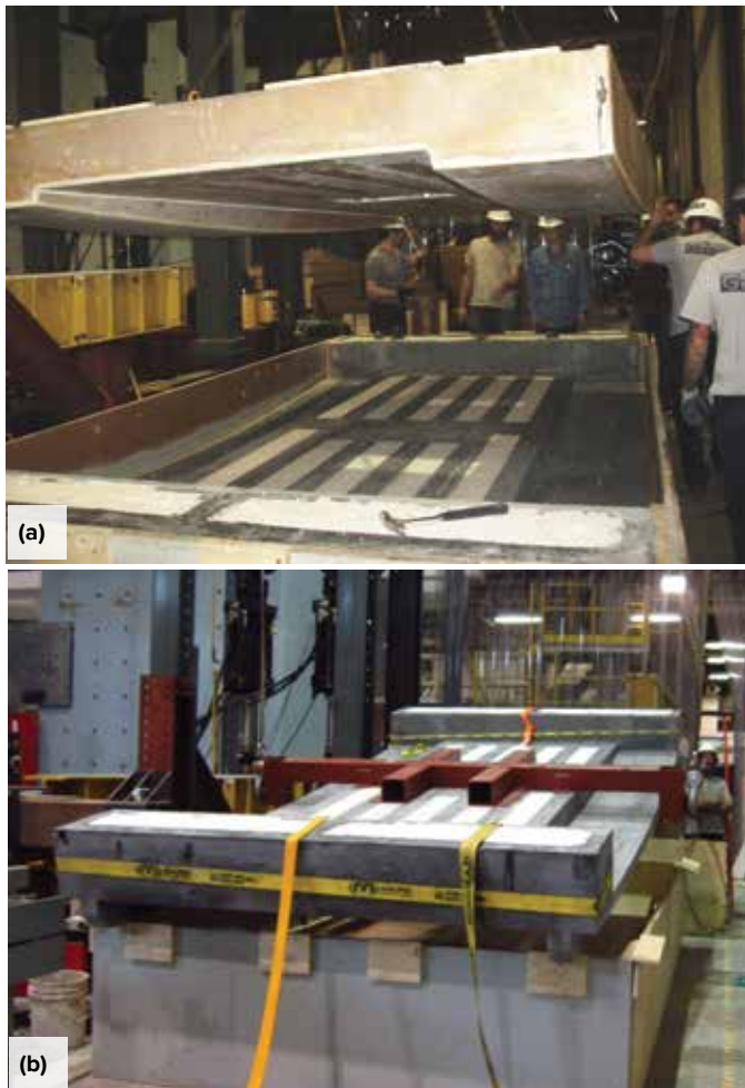
Fig. 3: The footbridge was cast upside down. The mold base held the urethane rubber liner shown in Fig. 2, and the mold was closed with a separate wooden insert that formed the curved and ribbed bottom surfaces of the footbridge: (a) the insert is removed from the mold base, exposing the bottom concrete surfaces and the expanded polystyrene blocks indicated in Fig. 1; and (b) the footbridge was pulled from the mold using straps and anchors, and a steel frame was attached in preparation for flipping the completed structure
