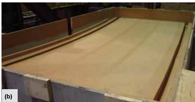
Fig. 2: The footbridge mold was designed to provide formed surfaces on all exposed faces: (a) a wooden insert was fabricated in the shape of the deck wearing surface and curbs; and (b) the insert was used as the master to cast the urethane rubber liner used for production of the footbridges
